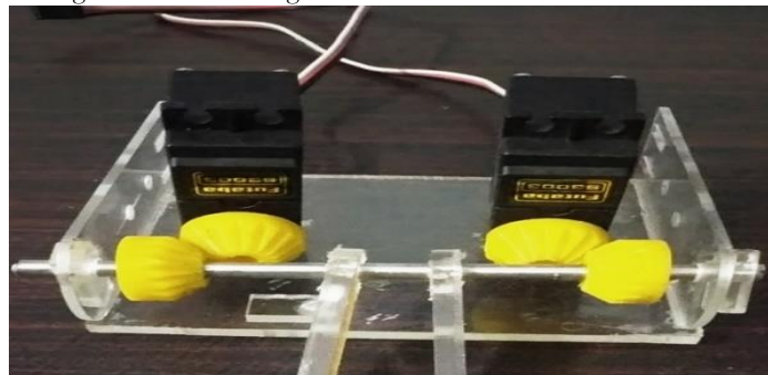
Figure 6. Bevel gear assembly with servo motors
